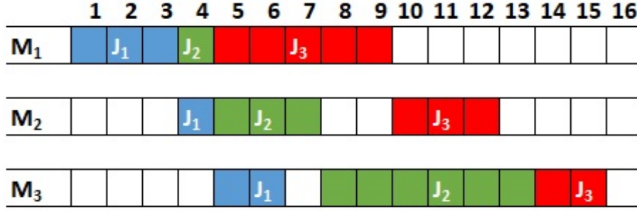
Figure 1.4: Gantt chart for the permutation flow shop example
